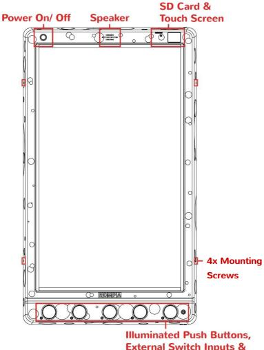
**External Switch Inputs & Microphone Input**
