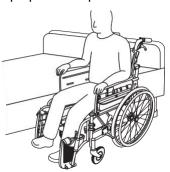
4. Unlock the armrest lever and flip upwards
