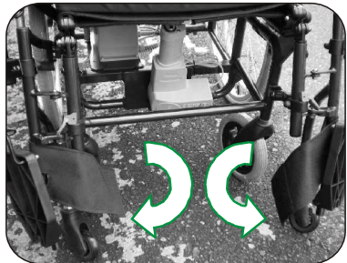
C2. Unlock the footrest (as left image), and footrest can be moved outside (as right image).
