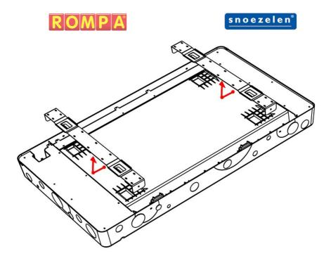
Hold the panel where you would like it to be mounted ensuring it is level. Whilst in position mark where the centre of the bracket mounting holes are on the wall. Do this for all 4x bracket mounting holes.
