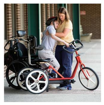
Transfers are made easy with the low step, flip-away loop handlebar and removable laterals.
