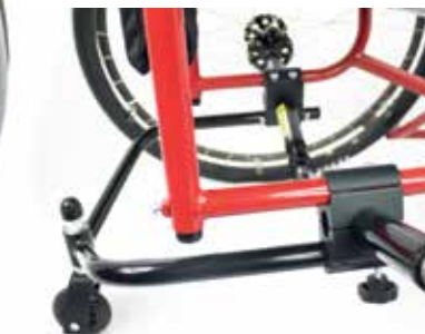
Adjustable COG and Quick release height adjustable Anti tip.
