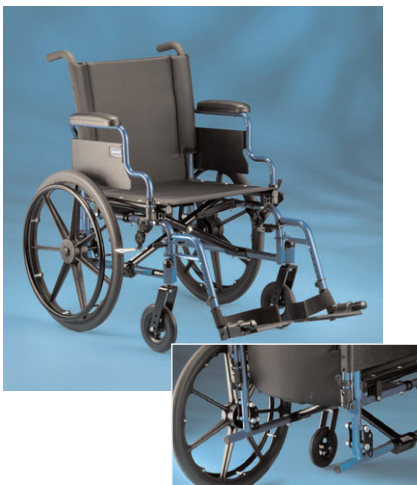
9000XT with offset axle and adjustable angle caster will allow additional seat-to-floor heights and increase seating and positioning capabilities. Offset axle offers center-of-gravity adjustment which increases maneuverability and stability.
