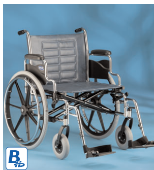
Heavy-duty package increases weight capacity to 450 lb. and consists of heavy-duty composite wheels with pneumatic tires with flat-free inserts and semi-pneumatic casters.
