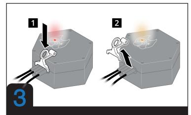
To activate the MeterDog, place the magnet as indicated for 30 seconds. Remove the magnet once the LED switches from Red to Orange.
