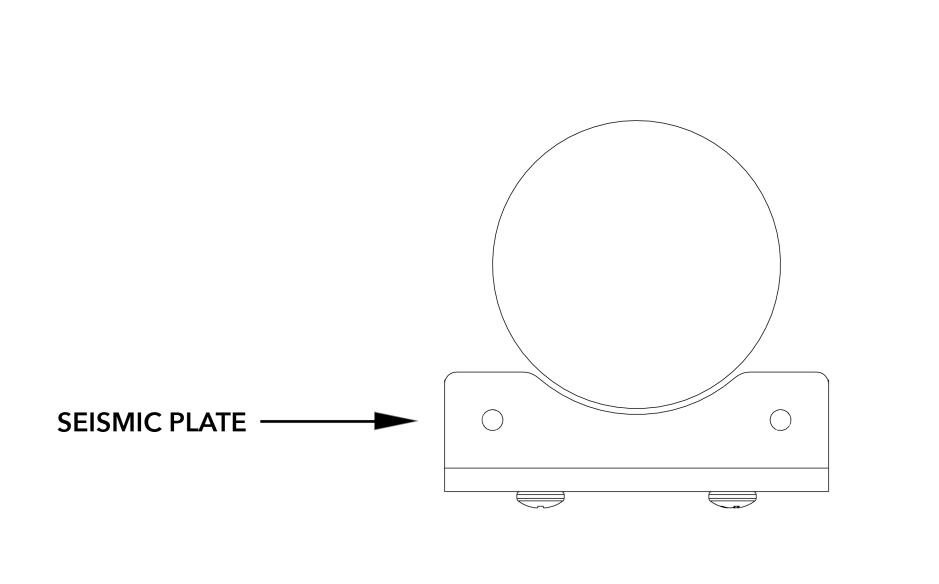
Place the seismic anchoring template on the floor where you want the booth and secure it in place with tape.
