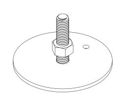
To level the base, spin the feet until each of the two built in levels show the bubble in the middle of the two lines. Press on the base to test that it is stable on all sides.
