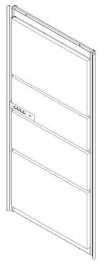
**Note:** The back wall will have the electrical outlet and motion sensor. Be careful not to damage the sensor during installation. Make sure the wires at the bottom and top of the back wall are taped securely and do not pinch the wires between the base when placing the back wall on the base.
