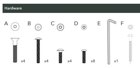
**Note:** (F) Seismic Hardware is optional for use with seismic install only.
