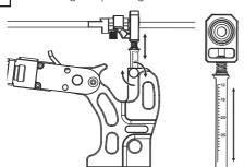
**6.6** Use an abrasive thickness compensator when working with abrasives of different thicknesses.
