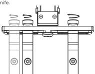
**6.2** The clamps must fit tightly to the knife.
