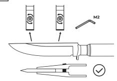
**6.3** The cutting edge of the knife should be parallel to the clamping frame.
