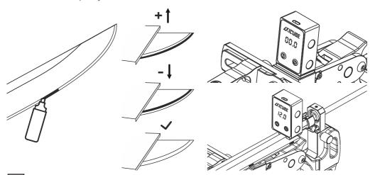
**6.10** Flip the knife, after sharpening one side.
