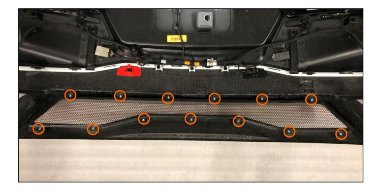
INSTALL U NUTS LOCATED IN HARDWARE BAG ONTO CARBON DIFFUSER GRILL MOUNTING TABS (ALIGN U CLIP THREADS WITH DIFFUSER TAB HOLES)
