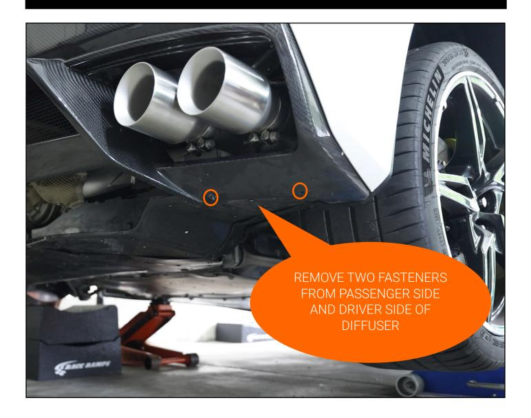
REMOVE 14 T15 TORX FASTENERS AND TWO 7MM FASTENERS ON THE OUTSIDE EDGE (FASTENERS LOCATIONS CIRCLED IN ORANGE)
