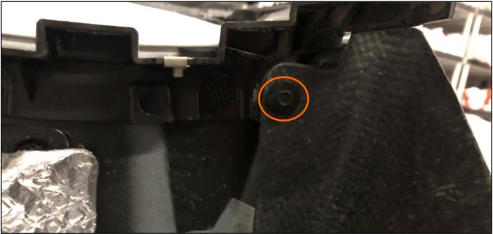
REMOVE 18 PLASTIC CLIPS THAT FASTEN OEM DIFFUSER TO BUMPER COVER THEN SEPARATE DIFFUSER FROM BUMPER COVER (SAVE CLIPS)
