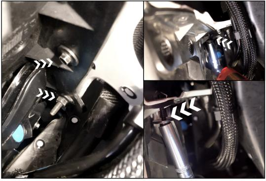
REMOVE FOUR T15 TORX FASTENERS FROM LOWER EDGE OF DIFFUSER WHERE IT FASTENS TO THE UNDERTRAY
