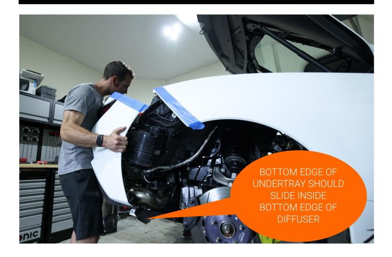
DOUBLE CHECK BUMPER COVER SEAMS ARE ALIGNED CORRECTLY AND REINSTALL THE 14 T15 TORX FASTENERS AND TWO 7MM FASTENERS ON THE OUTSIDE EDGE (FASTENERS LOCATIONS CIRCLED IN ORANGE)
