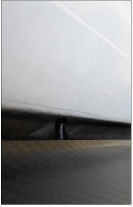
WARNING: BE CAREFUL NOT TO BEND THE CARBON FIBER SO MUCH THAT THE SURFACE IS GREATLY DISTORTED TO PREVENT CRACKING THE CLEAR COAT ALONG THE SEAM OF THE SKIRT. THE SKIRT IS EXTREMELY STRONG BUT THE CLEAR COAT IS MORE SUSCEPTIBLE TO CRACKING WHEN BENT AT EXTREME ANGLES. ALTERNATIVELY SOME PEOPLE USE A PICK AND TRY TO PUSH THE CLIPS IN FROM THE INBOARD SIDE OF THE VEHICLE.
