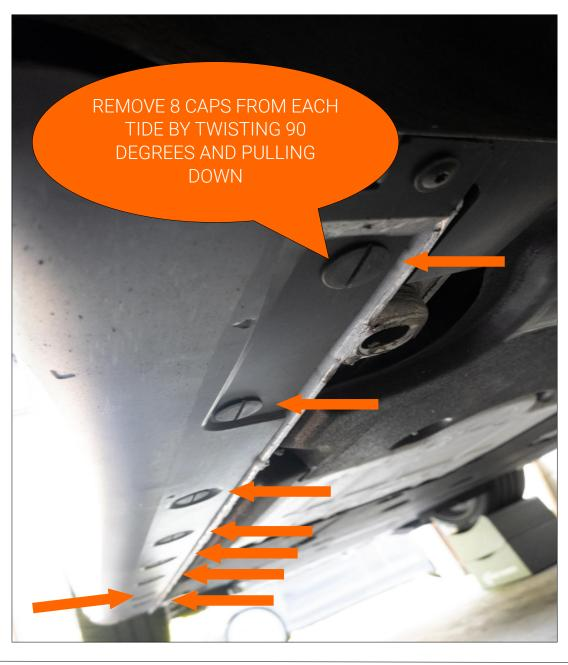
REMOVE THE OEM SIDE SKIRT. START AT THE BACK AND WORKING FORWARD BECAUSE OF A SMALL TAB AT THE LEADING EDGE OF THE SIDE SKIRT.
