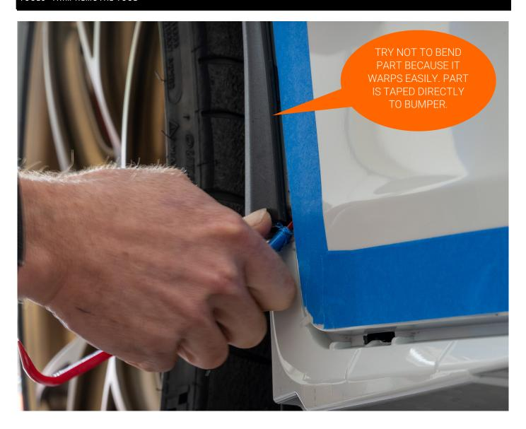
USING A GUMMY WHEEL CAREFULLY REMOVE TAPE RESIDUE FROM AREA HIGHLIGHTED IN ORANGE BELOW
