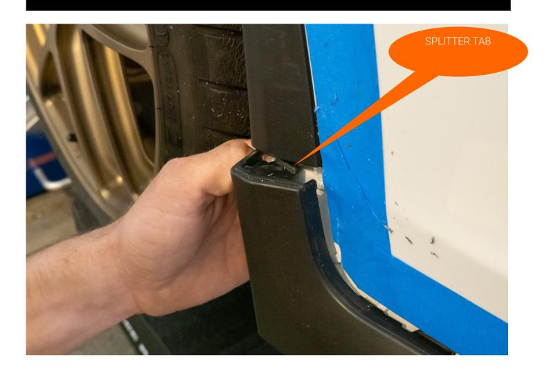
FREE SPLITTER TABS FROM BUMPER USING TRIM REMOVAL TOOL WORKING FROM ONE END TO THE OTHER. SPLITTER TABS ARE SPACED ROUGHLY 6 INCHES APART. CAREFULLY FREE THE TABS BY PUSHING DOWN ON THEM WITH THE TRIM TOOL.
