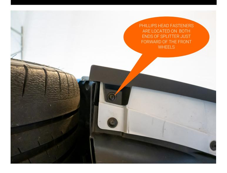
REMOVE OEM SPLITTER BY STARTING ON EITHER END AND PULLING SPLITTER AWAY FROM BUMPER UNTIL THE FIRST TAB IS FREE AS SHOWN BELOW.
