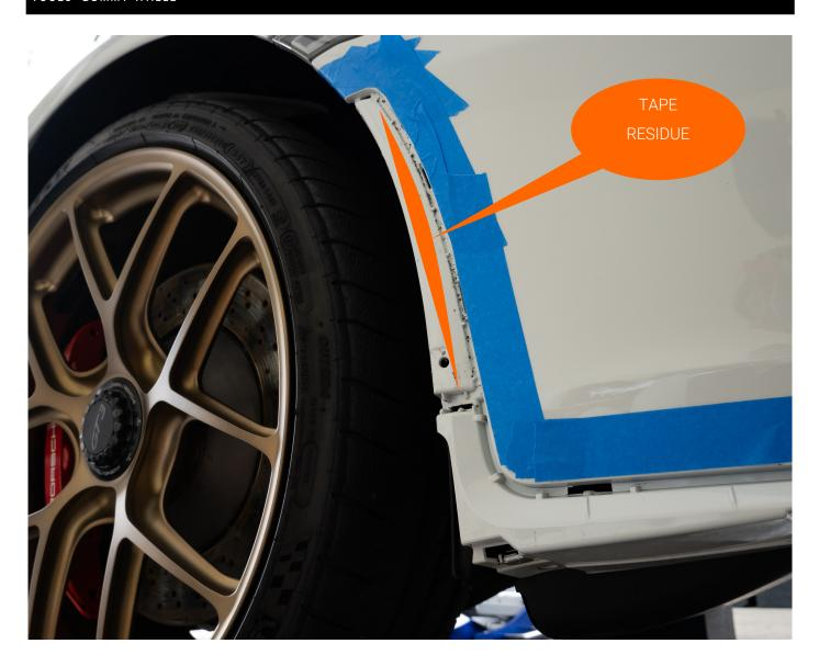
CLEAN SURFACE AND APPLY ADHESION PROMOTER TO UPPER SPLITTER PART MOUNTING AREA HIGHLIGHTED IN ORANGE BELOW
