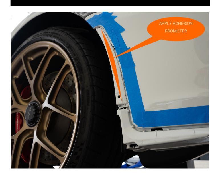
INSTALL CARBON UPPER SPLITTER PART BY FIRST REMOVING THE RELEASE LINER FROM THE TAPE
