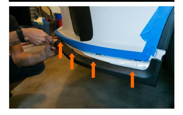
REMOVE UPPER SPLITTER PART USING TRIM REMOVAL TOOL TO SEPARATE PART FROM THE BUMPER STARTING AT THE BOTTOM WORKING YOUR WAY TO THE TOP.
