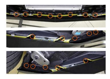
Reinstall the central section of the undertray and the 8x 7mm fasteners circled in orange
