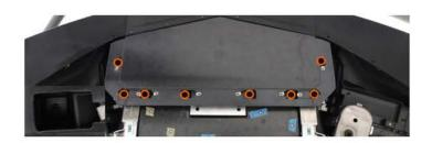
Remove the 4x 7mm fasteners that fasten the 3x splitter pieces together
