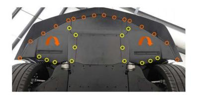
Remove the 9x 7mm fasteners circled in orange and remove this section of the undertray.
