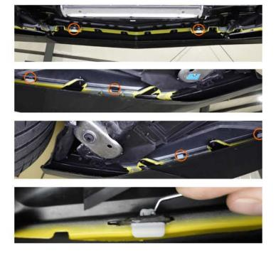
Remove the 18x 7mm fasteners circled in orange.
