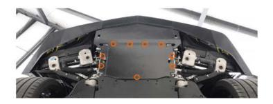
Reinstall the undertray side pieces and the 16x T15 fasteners circled in yellow.
