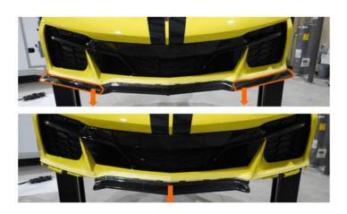
First install center section of RSC carbon fiber splitter by aligning; the 2 tabs indicated with the orange arrows with slots in the bumper.
