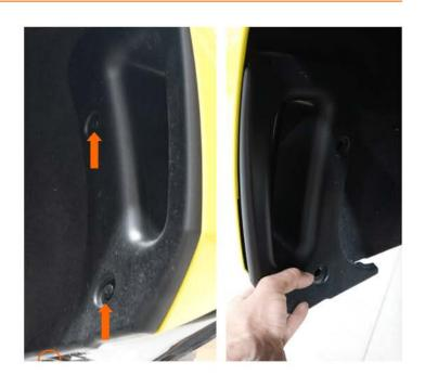
Remove T15 fastener from fender liner.
