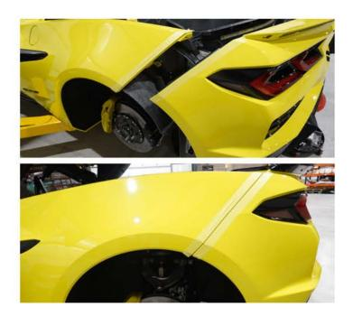
Double check bumper cover seams are aligned correctly and reinstall the 16x T15 fasteners along the rear edge of the bumper.
