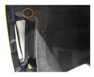
Reinstall rear mud flaps by pushing clips into slots working from top to bottom.
