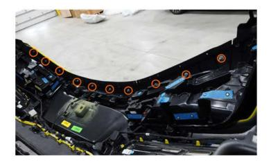
Position bumper cover about 6-8 inches from the rear of car and plug in the 3x electrical connectors circled in orange (1 large white, 1 small back, and 1 large black)
