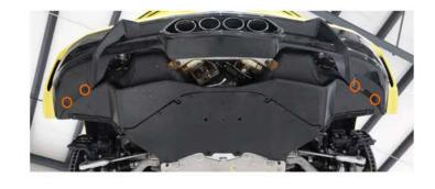
Open decklid and remove 16x T15 torx fasteners from the bumper (fasteners locations circled in orange)
