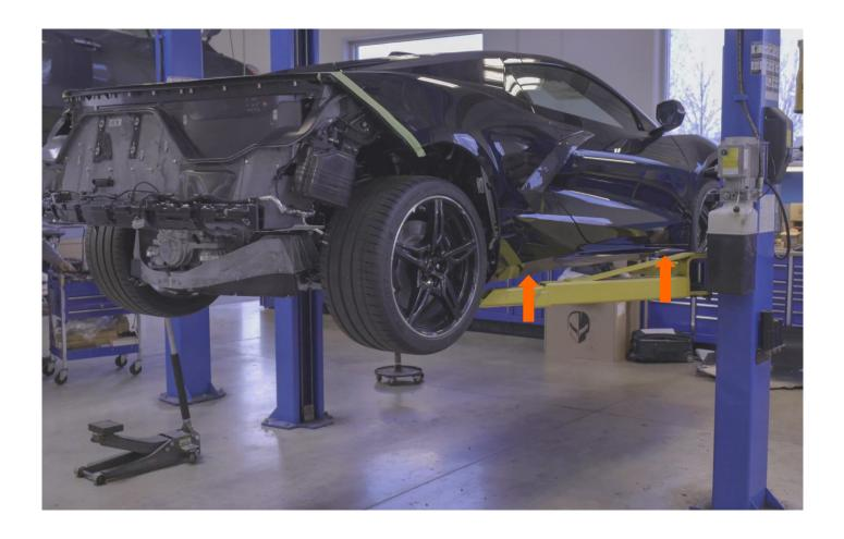
REMOVE THREE 7MM FASTENERS FROM UNDERSIDE OF ROCKER PANEL -REPEAT ON OTHER SIDE-
