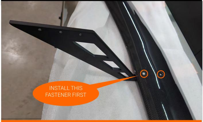
WARNING: Stanchions are machined out of aluminum to save weight. Hardware is stainless steel for corrosion resistance. The stainless steel fastener can easily damage the aluminum threads in the stanchions if cross threaded. Carefully hand thread bolts into stanchions only DO NOT TIGHTEN YET
