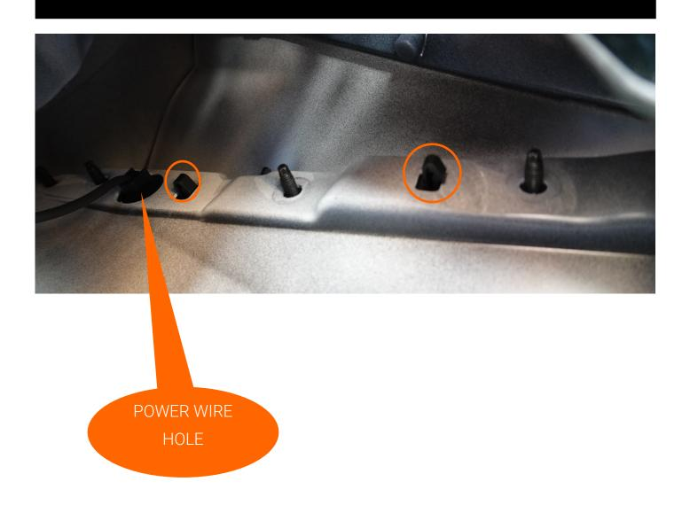
REINSTALL THE TWO T30 TORX FASTENERS ON THE DOOR HANDLE AND THEN THE FOUR 10MM NUTS ON THE INSIDE OF THE DOOR PANEL -FASTENER LOCATIONS CIRCLED IN ORANGE-
