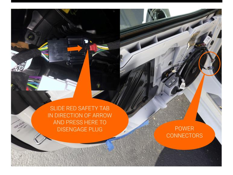
PEEL SOUND BARRIER SHIELD BACK TO GET ACCESS TO DOOR HANDLE FAS\_ TENERS AND DOOR HANDLE POWER CONNECTOR
