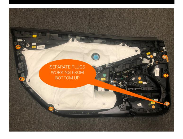
DOOR PANEL POWER CONNECTOR REMOVAL INSTRUCTIONS -INSTRUCTIONS WORK FOR BOTH CONNECTORS-
