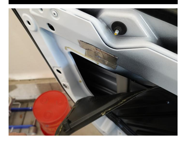
UNPLUG DOOR HANDLE POWER CONNECTOR AND REMOVE CLIP THAT FASTENS WIRE TO THE INSIDE OF DOOR
