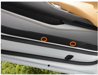
REMOVE DOOR PANEL USING TRIM REMOVAL TOOL TO SEPARATE DOOR PANEL PLUGS FROM DOOR AND THEN UNPLUG POWER CONNECTORS BEFORE REMOV\_ING COMPLETELY -SEE STEP 4 FOR POWER CONNECTOR INSTRUCTION—
