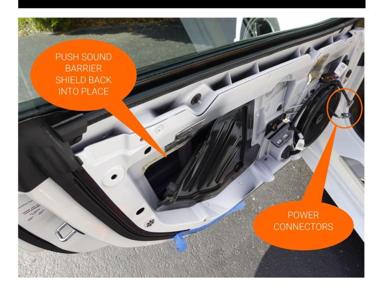
REINSTALL DOOR PANEL BY POSITIONING TOP EDGE OF THE DOOR PANEL OVER THE AREA HIGHLIGHTED IN ORANGE! PRESS DOWN UNTIL FULLY SEATED AND ALIGN DOOR PANEL PLUGS WITH HOLES AND PRESS INTO PLACE TOOLS...
