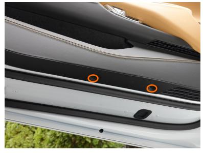
REMOVE FOUR 8MM FASTENERS FROM LOWER SIDE INTAKE VENT AND REMOVE OEM PART - FASTENER LOCATIONS ARE CIRCLED IN ORANGE-
