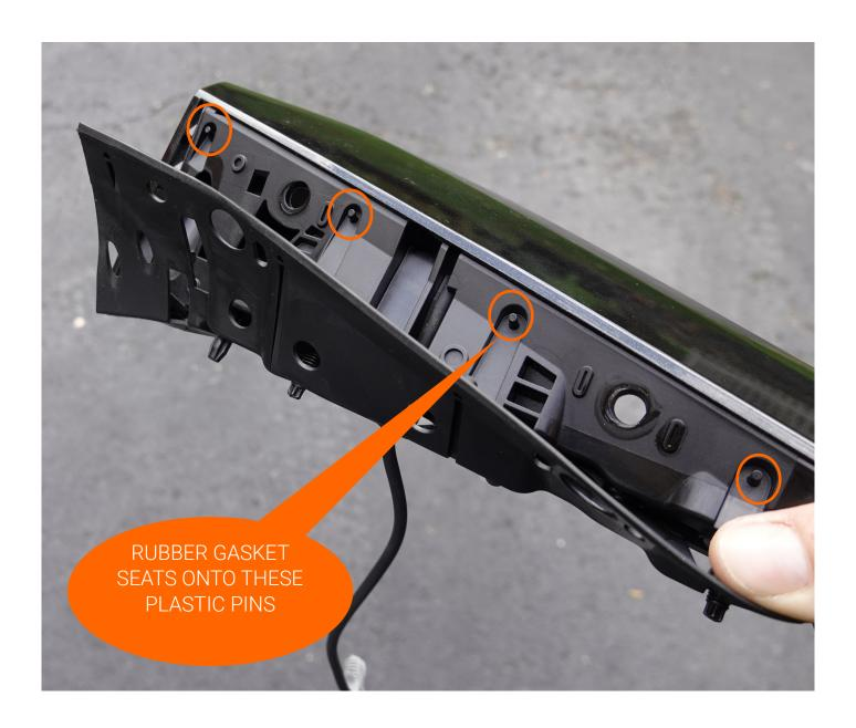
REINSTALL DOOR HANDLE BY FIRST FEEDING POWER CONNECTOR THROUGH THEN PUSHING CLIPS INTO PLACE -CLIPS ARE CIRCLED IN ORANGE-TOOLS...NONE
