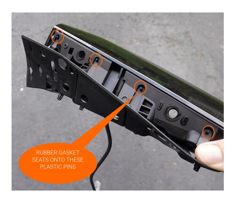
REMOVE FOUR T20 TORX FASTENERS FROM DOOR HANDLE HOUSING -FASTENER LOCATIONS CIRCLED IN ORANGE-
