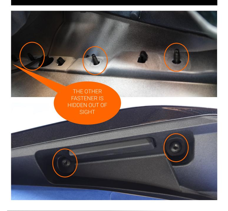
REMOVE DOOR HANDLE BY DISENGAGING THE CLIPS CIRCLED BELOW WHILE HOLDING DOOR HANDLE FROM THE OUTSIDE
