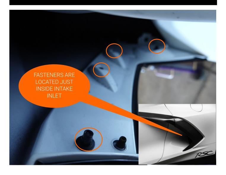
INSTALL CARBON FIBER LOWER INTAKE VENT AND REINSTALL 8MM FASTEN\_ERS
