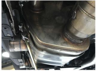
**Step 12:** Install the band straps over the center muffler and muffler mounting bracket and tighten the 6mm allen head.
