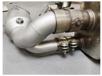
**Step 9:** Install the Soul Performance Products Sport Catalytic Converters into position, leave assembly loose to allow for adjustments later.
