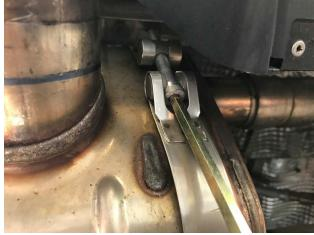
**Step 5:** Moving to the center muffler, using a 6mm allen drive loosen the band strap and slide it to the outside of the muffler.
