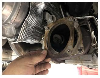
**Step 10**: Clean the flange on the turbo of any debris and reinstall the OEM metal gasket. You can use a copper gasket sealant to aid in this process.
