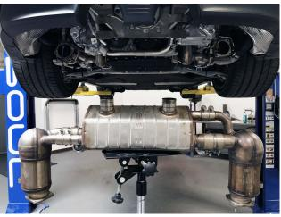
**Step 7:** Carefully slide the exhaust towards the rear of the car and gently lower it out being careful not to damage the studs on the turbo. (PSE Version Muffler Pictured)
