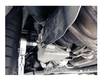
**Step 1:** With the car safely supported, using a T30 torx socket remove the (4) torx bolts that secure each heat shield to the turbos and catalytic converters.
