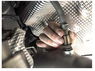
**Step 14:** Reinstall the oxygen sensors using anti seize and a 22mm wrench.
