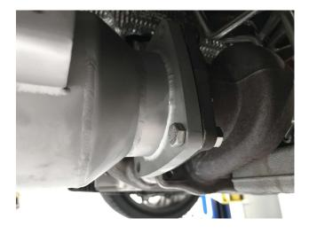
**Step 11**: Guide the exhaust and catalytic converters up and into position and tighten the hardware with the 4 nuts and 3 bolts provided. One nut will be placed on the factory stud on the turbo.
