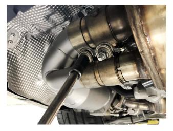
**Step 13:** Tighten the accuseal and torca clamp locking the center muffler and catalytic converters together.
