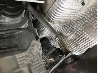
**Step 4:** Using a 22mm wrench loosen and remove both oxygen sensors. Be mindful of their positions (primary and secondary locations) and mark them if necessary to ensure that you re-install them in the correct position.
