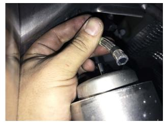
**Step 16**: Reinstall the factory vacuum hoses to the two valves on the PSE muffler.
