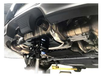
**Step 6:** Support the muffler with the help of a friend or a transmission jack. (PSE Version Muffler Pictured)
