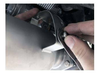
**Step 15:** Reinstall the factory heat shields onto your Soul Performance Products Sport Catalytic Converters.
