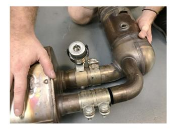
**Step 8:** Using a 15mm socket, loosen the accuseal clamp on the larger pipe and 13mm socket to loosen the torca clamp and slide the catalytic converter out.
