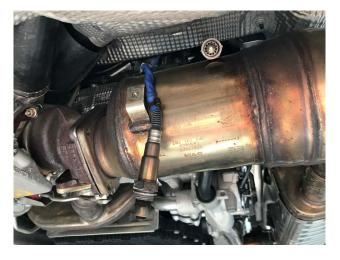
Avoid touching the exposed sensor as the oil in your hands can damage their ability to read correctly.
