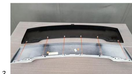
1. Plastikkappe lösen / *Release the plastic cap*
