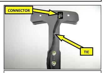
**2.** Open the tailgate to gain access to the third brake light bracket wiring and hardware. Cut the cable tie securing the harness and disconnect the brake light.
