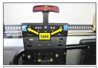
**21.** Use two pieces of painters tape to hold the Studs in position.
