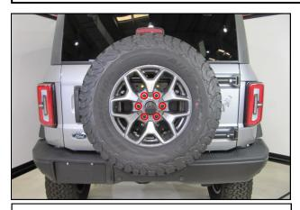
**1.** With the vehicle parked on a level surface remove the spare tire and set it aside.
