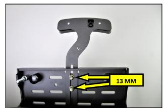
**18.** Torque the nuts to 14 lb. ft. Threadlocker is not to be used on these fasteners.
