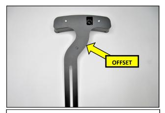
**16.** To help keep the third brake light centered with a repositioned Hub, RTR has included an Off Set Light Bracket. Transfer the Offset bracket onto the brake light and secure it using the hardware from the original bracket. Threadlocker is not to be used on these fasteners.
