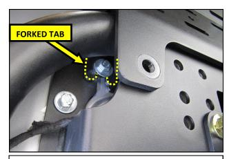
**11.** When properly fitted, the forked tabs will be between the tire carrier and the washers on the loosened bolts from step **9**.
