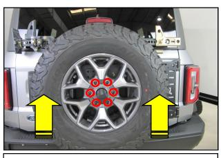
**25.** With the help of an assistant, carefully reinstall the spare tire onto the vehicle to avoid scratching and torque the lug nuts to 41 lb.ft.
