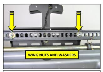
**23.** Secure the jack to the Mount using the supplied Wing Nuts and 3/8 Washers. Tighten the Wing Nuts Hand Tight. Threadlocker is not to be used on these fasteners.
