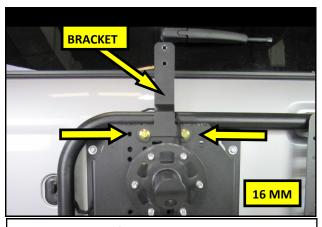
**4.** Remove the two flange bolts securing the lower bracket to the tire carrier and remove the bracket.
