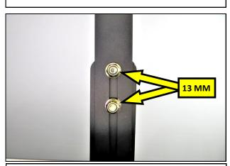
**3.** Remove the lock nuts securing the upper light bracket to the lower bracket. Remove the upper bracket, light and hardware and set them aside.
