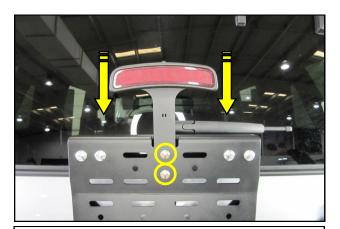
**13. INSTALL OPTION A:** Install the brake light and bracket onto the mount using the hardware removed in step 3.
