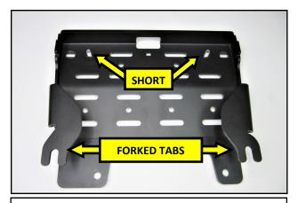
**5.** Insert the 3/4" (Short) Carriage Bolts into the Mount as shown, face down, with the forked tabs facing up .
