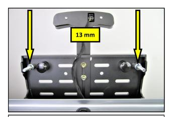
**22.** Tighten the Lock Nuts, final tight, to 15 lb.ft. Threadlocker is not to be used on these fasteners.
