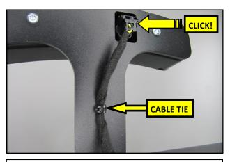
**19.** Reconnect the harness to the third brake light. Secure the wire harness to the Upper Brake Light Bracket using the supplied Cable Tie. Trim the excess length.
