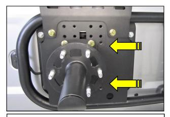
**15. INSTALL OPTION B:** The tire carrier hub can be repositioned to accommodate carrier mounted accessories.
