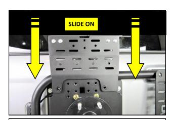
**10.** Slide the Mount onto the tire carrier as shown, with the forked tabs onto the loosened bolts from step **9**.
