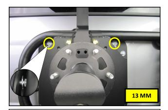
**9.** Loosen the two top tire carrier bolts approximately 1/4 inch.
