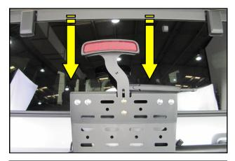
**17.** Install the brake light and Bracket onto the Mount using the hardware removed in step **3**.
