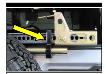
**28.** Install a handle keeper (not included) onto the jack handle to eliminate rattling during transportation.
