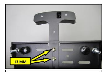
**14.** Torque the Lock Nuts to 14 lb.ft Threadlocker is not to be used on these fasteners.
