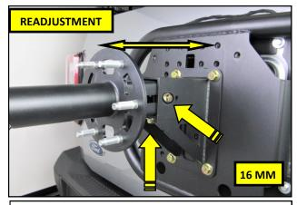
**27.** Loosen the 2 flange bolts on the tire carrier base and adjust as needed. Torque the flange bolts to 45 lb.ft. Reinstall the spare tire and re torque the lug nuts.
