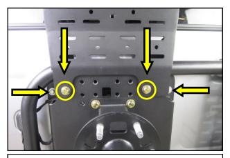
**12.** Use the supplied M12 Flange Bolts to secure the Jack Mount to the tire carrier and torque the Bolts to 45 lb.ft. Tighten the M8 bolts from step **9** to 30 lb.ft.
