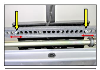
**20.** With the help of an assistant, lift the jack up and onto the Jack Mount Studs a shown. Adjust the Stud positioning left or right to fit the hole spacing of the Jack.
