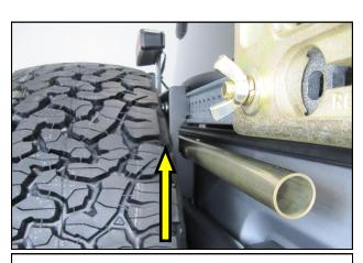
**26.** Check the tire to Jack Mount clearance. When properly installed, the tire will be in contact with the Mount but should not require forcing the tire onto the hub. Readjust if necessary.
