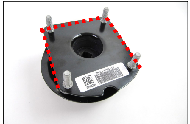
14. For 2011-2014 vehicles with the square type strut mount, the steel spacers will be needed.
