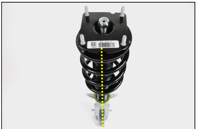
16. Transfer the OEM upper strut mount and spacer onto the RTR Coilover assembly and use the supplied nut to secure the mount onto the piston rod and torque to 46 lb.- ft. Align the arrow with the strut clevis as shown.
