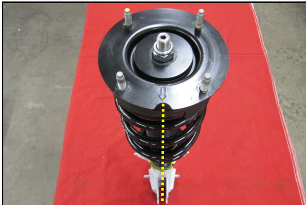
13. Transfer the OEM upper strut mount onto the RTR Coilover assembly and use the supplied nut to secure the mount onto the piston rod and torque to 46 lb.- ft. Align the arrow with the strut clevis as shown.
