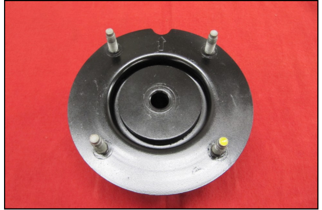
12. Remove the piston rod nut from the strut and remove upper strut mount. Inspect the bearing for wear and replace if necessary.
