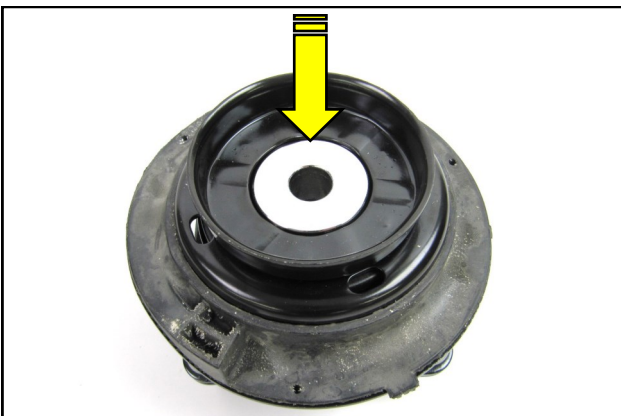
15. Insert the steel spacer into the bottom of the strut mount as shown.
