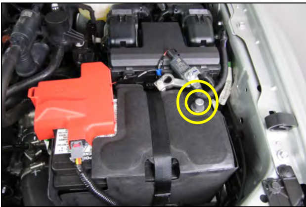
1. Raise the vehicle hood and disconnect the negative terminal on the battery.
