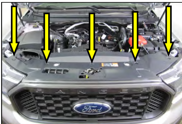
3. Remove the 5 plastic rivets in the core support cover.
