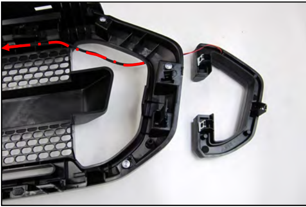
17. Route the wiring harness through the front of the Grille and insert the LED or Insert into the RTR grille. The LEDs and Inserts are side specific and are marked accordingly on the back side.
