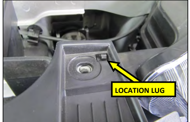
10. With the grille bolts removed, lift up on the grille tabs and pull the grille slightly forward to clear the location lugs.
