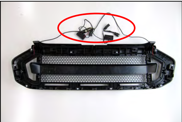
19. Install the second LED or Insert into the grille and lay the wiring harnesses up and away from the grille as shown.
