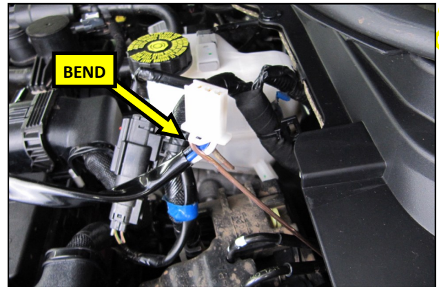
32. Route the connector side of the main harness along the fender towards the firewall. Bend the hanger over the harness as shown. HINT: Wrapping the connector and wire with electrical tape will allow the connector to pass through the grommet with greater ease.
