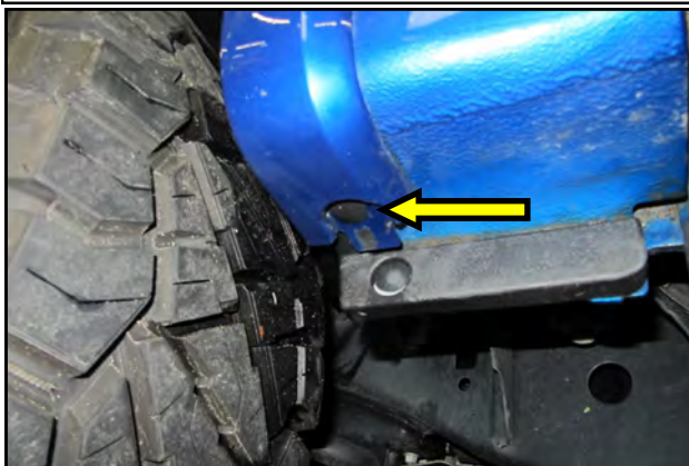
3. Starting at rear of the flare, remove the plastic fastener securing it to the rocker panel.
