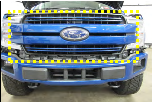
15. Slide the OEM grille and shutter assembly forward and out of the vehicle.
