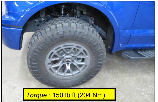
52. Reinstall the wheels and tires and lower the vehicle onto the ground. Torque the lug nuts to 150 lb.-ft
