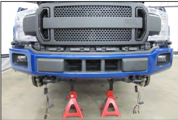
39. Remove the bungee cord and fully insert the RTR Grille assembly into the vehicle.
