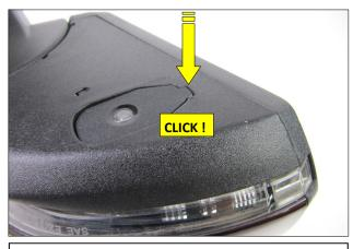
**7.** Press firmly onto the back of the Lamp, compressing the locking tab, until a distinct click is heard indicating full engagement of the locking tab.
