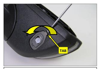
**2.** Using a jewelers screwdriver or equivalent, carefully depress the locking tab in the puddle lamp and pry it out of the housing.
