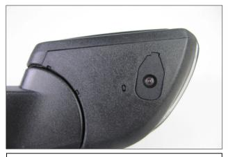
**8.** Underside view of mirror assembly with properly installed Puddle Lamp.
