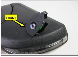
5. Using both hands, carefully guide the front of the Lamp into the housing while pulling the rear of the Lamp slightly upward.
