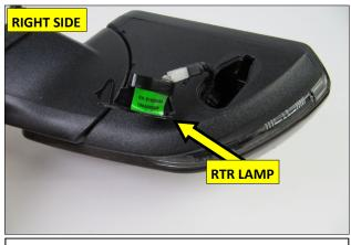
**4.** Connect the respective RTR Puddle Lamp to the harness. **NOTE:** The Right Hand Lamp is marked in Green and the Left Hand Lamp is marked in Blue.
