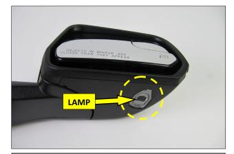
**1.** Disconnect the Negative terminal of the Battery. Locate the puddle lamp in the bottom of the mirror housing. **NOTE:** The mirror assembly has been removed for illustrative purposes only.
