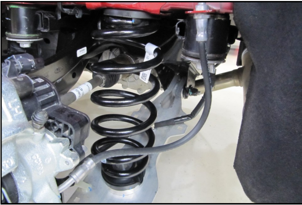
41. Push down on the control arm and reinstall the spring. Ensure that both coil ends are properly positioned on the isolators.
