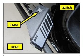
**7.** Using a 5MM Allen socket or equivalent, secure the Foot Rests to the hinges with the supplied bolts. Torque the Bolts to 22 lb.ft.
