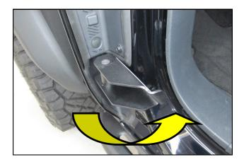
**8. NOTE:** A key design feature of the RTR Foot Rests is that they can be easily folded inboard, when needed, for additional clearance.
