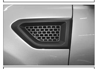
**9**. Insert the RTR vent into the vehicle fender as shown. Repeat steps **1-9** on the opposite side of the vehicle.
