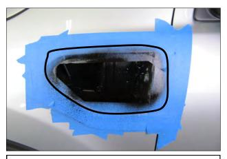
**7. Install Option:** Place additional painters tape around the fender opening and spray paint the inner fender black. This will conceal high contrast paint colors behind the RTR vent.
