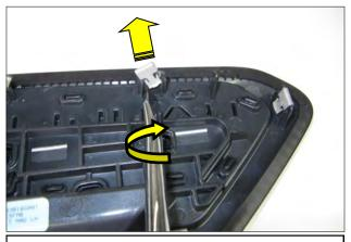
**5**. Using a 5/16" standard blade screwdriver or equivalent, carefully pry the clips off of the OEM vent.
