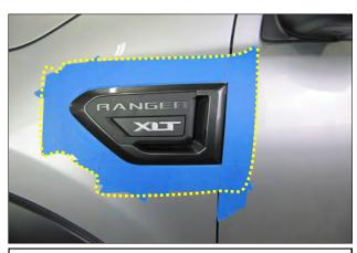
**1.** Prepare the vehicle for OEM vent removal by placing a protective layer of painters tape on the fender, as shown.
