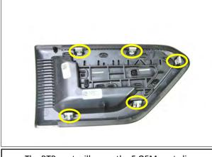
The RTR vent will reuse the 5 OEM vent clips.
