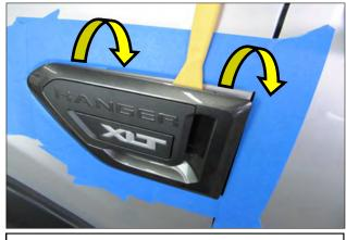
**2.** Using a no-scratch pry tool, carefully pry the OEM vent out of the fender.
