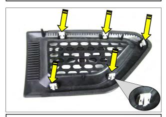
**6.** Transfer the OEM clips from step 6. onto the RTR vent as shown, with the large protrusion facing outwards.
