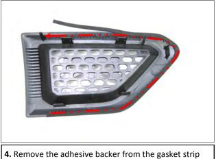
**4.** Remove the adhesive backer from the gasket strip and apply it to the edge of the RTR vent as shown.
