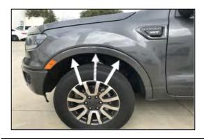
**5.** Using Philips head screwdriver remove factory wheel arch fasteners in the three shown locations. Install the screw plugs provided in the hardware kit into the shown locations.
