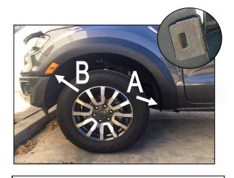
7. Apply upward tension on Fender Flare to the vehicle fender when installing the large U clip in location A and the small U clips in location B. Slide the clips over the Fender Flare and the inner wheel arch lip in the two locations shown. Position the clip so that the barb in the clip locates in the slot of the Fender Flare.
