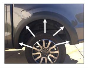
**15.** Place Fender Flare on the vehicle into the position of best fit. To secure the Fender Flare to the vehicle body, apply upward tension on Fender Flare to the vehicle fender when installing the large U clips. Slide the clips over the Fender Flare and the inner wheel arch lip in the five locations shown. Position the clip so that the barb in the clip locates in the slot of the Fender Flare.
