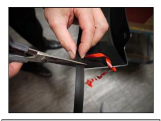
**9.** Attach the included rubber seal to the Front 1/4 Fender Flares. Peel back 2" of the adhesive backing and position on the 1/4 Fender Flare. Attach the seal to the 1/4 Fender Flare, peeling back a few inches at a time. Ensure pressure is used to secure rubber seal to 1/4 Fender Flare edge. Attach rubber seal along all areas the 1/4 Fender Flare will make contact with the vehicle. Trim excess rubber seal and discard.
