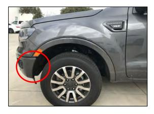
**10.** Clean the bumper body where the 1/4 Fender Flares will make contact. Ensure bumper area are dry prior to install. Turn the tires outward for Fender Flare installation.
