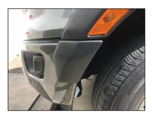
**12.** Starting at the front of the 1/4 fender flare, remove tape liner from rubber gasket. Ensure rubber gasket is not tucking into flare and flush neatly against the bumper body. Ensure all fixing points are tight and secure. Repeat install steps for the opposite side of the
