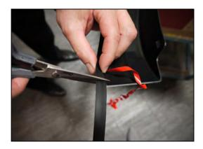
13. Attach the included rubber seal to the Fender Flares. Peel back 2" of the adhesive backing and position on the Fender Flare. Attach the seal to the Fender Flare, peeling back a few inches at a time. Ensure pressure is used to secure rubber seal to Fender Flare edge. Attach rubber seal along all areas the Fender Flare will make contact with the vehicle body. Trim excess rubber seal..
