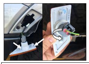
**3.** Removal of the turn signal is required for installation of front Fender Flares. Pull back the inner wheel well liner to locate the turn signal body and wiring. Remove the turn signal from the vehicle body by squeeze the lower tab on the back of the turn signal body. Carefully turn the wiring harness counter clockwise and remove the bulbwiring harness from the turn signal body.
