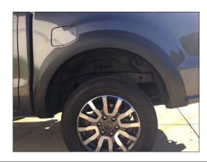
**16.** Starting at the front of the rear fender flare, remove tape liner from rubber gasket. Ensure rubber gasket is not tucking into flare and flush neatly against the bumper body. Ensure all fixing points are tight and secure. Repeat install steps for the opposite side of the
