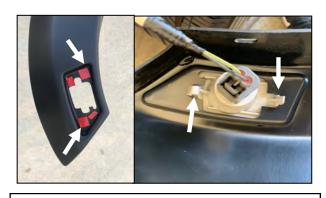
**4.** Apply the provided tape squares 3 per side to the turn signal recess, cutting of the tapes will be required per image. Remove the tape liner, install the turn signal body into the recess in the front Fender Flares. Ensure the tabs in the back of the turn signal body snap into the Fender Flare recess pocket. Apply firm pressure across the turn signal once in place to achieve tape wet out. Reinstall the bulb-wiring harness to the turn signal body.
