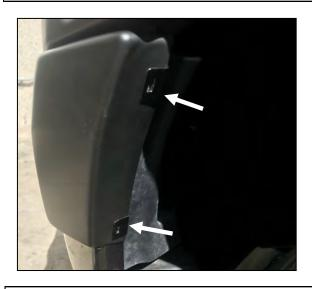
11. Apply tension to 1/4 Fender Flare to the vehicle bumper when installing the U clip in locations noted above. Slide the clips over the 1/4 Fender Flare and the inner bumper arch lip in the two locations shown. Position the clip so that the barb in the clip locates in the slot of the 1/4 Fender Flare.
