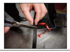
1. Attach the included rubber seal to the Fender Flares. Peel back 2" of the adhesive backing and position on the Fender Flare. Attach the seal to the Fender Flare, peeling back a few inches at a time. Ensure pressure is used to secure rubber seal to Fender Flare edge. Attach rubber seal along all areas the Fender Flare will make contact with the vehicle. Trim excess rubber seal and discard.
