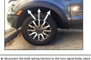
**6.** Reconnect the bulb-wiring harness to the turn signal body, place the Fender Flare onto the vehicle into position of best fit. To secure the Fender Flare to the vehicle body, install the provided screws and washers into the screw plugs in the three shown locations
