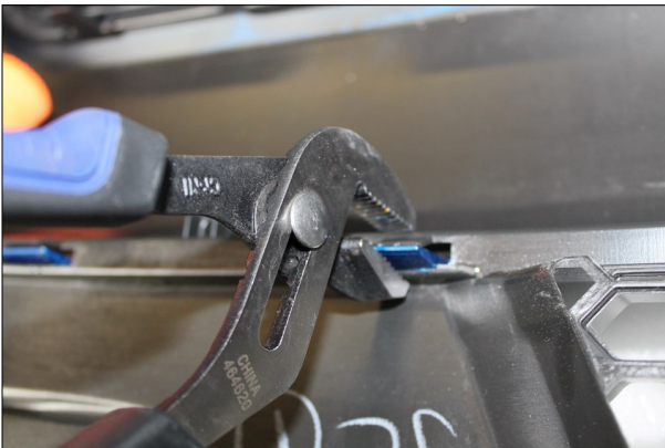
19. Using a combination of slip joint pliers and a large flat blade screw driver, depress the cover tabs one by one, from left to right and remove the upper grille.
