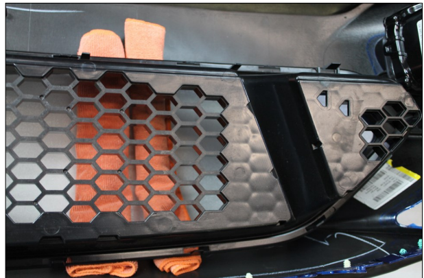
20. HINT: Using rolled shop towels to separate the grille from the cover will prevent the tabs from re-engaging the grille.
