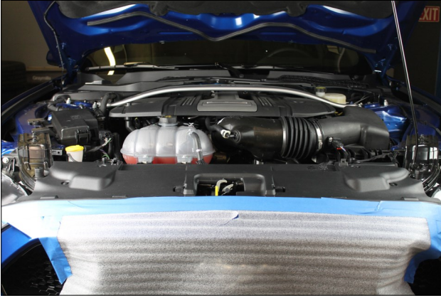
11. RTR recommends applying a protective film or a fender cover over the bumper for paint protection.
