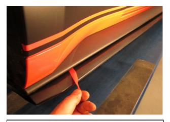
5. Peel the ends of the red plastic backing off of the Adhesive Strips on the RTR Rocker Splitter and lift into place on the vehicle.
