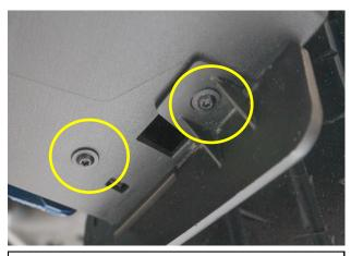
1. Using a T20 Torx bit, remove two Torx screws from the bottom of the splash shield.
