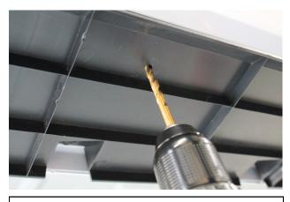
7. Using the holes in the RTR Rocker Splitter as a guide, drill four 1/4" holes in the OEM rocker panel.
