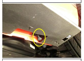
3. Remove the eight plastic clips securing the OEM rocker panel. These will not be reused.
