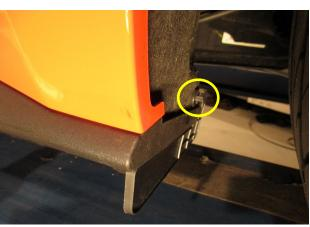
2. Remove one plastic rivet from the inside of the wheel well and remove the splash shield.
