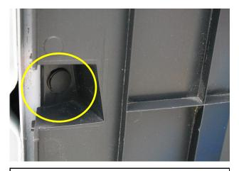
6. Install the eight provided Plastic Rivets into the factory hole locations. Once the Plastic Rivets are installed, peel the remaining red plastic backing off and firmly press the RTR Rocker Splitter against the OEM rocker to adhere.
