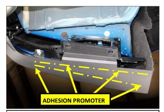
3. Using a mild soap and water solution, clean the OEM plastic of any and all debris. When completely dry, prepare the surface with the supplied Adhesion Promoter.
