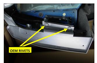
5. Carefully position the RTR Quarter Splitter and align the holes for the OEM rivets. Reinstall the OEM rivets, then press firmly onto the Adhesive Strip section.
