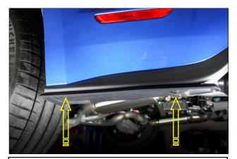
7. Install two of the supplied Plastic Rivets into the drilled holes in the valance.
