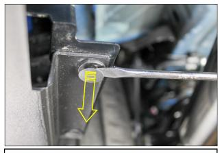
2. Using a flat tip screwdriver or equivalent, carefully pry out the center post and remove the rivets. Set the rivets aside – they will be reused in this installation.
