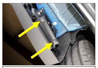
1. From underneath the vehicle, directly behind the rear tire, locate the OEM rear valance corner rivets. (Drivers side shown)
