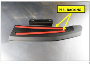
4. Peel the plastic backing off of the Adhesive Strips on the RTR Quarter Splitter.
