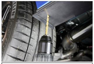
6. Using the holes in the RTR Quarter Splitter as a guide, drill two 1/4" holes in the OEM valance.
