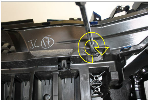
17. Using a large flat blade screw driver, depress the cover tabs one by one, from left to right and remove the center support.
