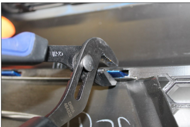
19. Using a combination of slip joint pliers and a large flat blade screw driver, depress the cover tabs one by one, from left to right and remove the lower grille.
