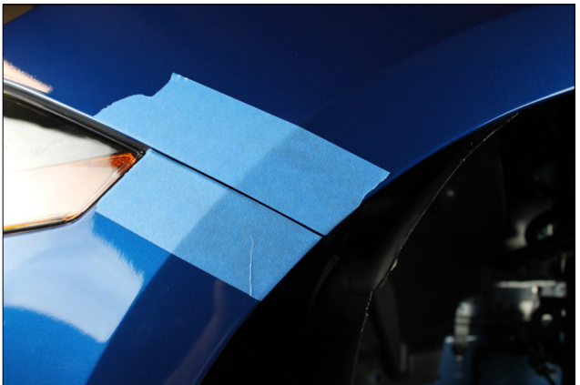
8. RTR recommends using painters tape as protection for areas susceptible to abrasion during disassembly and assembly.
