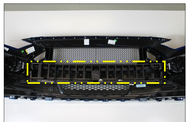
16. Remove the center support from the bumper assembly using the following steps.
