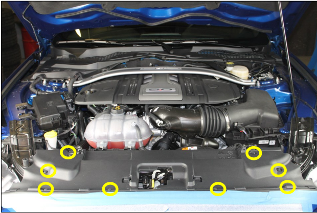
23. With the help of an assistant, lift the bumper cover back onto the vehicle and secure it using the OEM hardware. Reinstall the core support cover using the plastic rivets.
