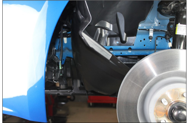
6. Pull the fender liners away from the bumper cover and tuck them behind the brake rotor.
