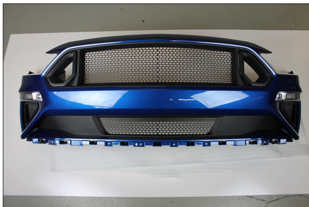
22. Inspect the RTR Lower Grille installation from the front of the bumper cover assembly and confirm all tabs are fully seated.
