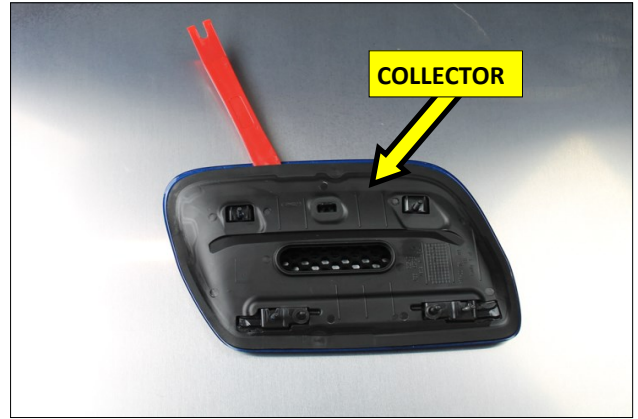
6. Using a Plastic, No Scratch, Pry tool, separate the collector from the hood vent.
