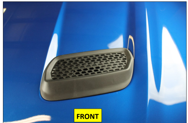
10. Install the RTR Hood Vent as shown, with the raised edge towards the front of the vehicle. Carefully press down to engage the factory tension clip.
