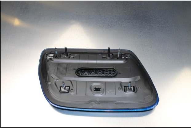
5. On a work bench, use a shop towel to prevent scratching and turn the vent up side down.
