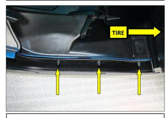
4. From the inside, remove the three small diameter plastic rivets at each side of the OEM front lip. Remove the OEM front lip and set it aside.
