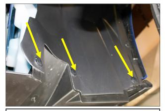
9. With the fender liner on the outside of the pan, reinstall the three rivets on both sides of the vehicle.
