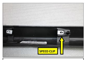
5. Transfer the speed clips from the OEM front lip onto the RTR Front Lip Spoiler. A small screwdriver or pick can ease removal of the speed clips.
