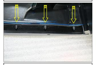
7. Reinstall the three small diameter plastic rivets on each side.
