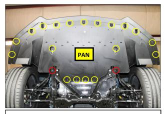
1. From underneath the vehicle remove the 19, 7mm head screws from the pan, marked in yellow and the two plastic rivets marked in red.
