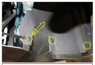
2. Remove the three remaining plastic rivets inside each wheel well. The pan can now be removed from the vehicle.
