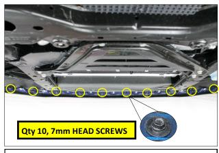
3. Remove the 10, 7mm head screws securing the OEM front lip.
