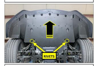
8. Reinstall the pan back onto the vehicle, leading edge first, then secure it using two OEM rivets at the rear.
