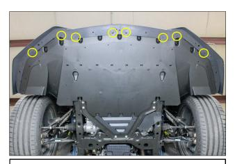
11. Install the eight Short RTR screws into the remaining eight open holes in the RTR Front Lip Spoiler.
