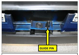
6. Slide the RTR Front Lip Spoiler onto the bumper using the three guide pins to locate. Starting from the edges and working towards the center, reinstall the 10 OEM screws to secure the RTR Front Lip Spoiler.
