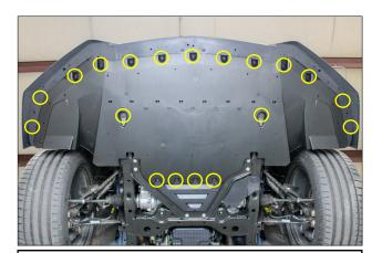
10. Reinstall the 19 OEM screws in the locations marked in yellow.
