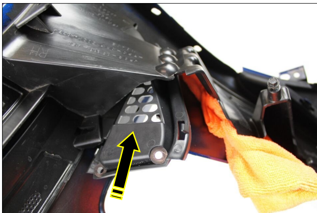
21. Insert the RTR Bumper Vent into the bumper cover and remove the shop towel.
