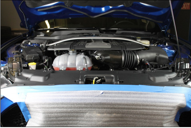
11. RTR recommends applying a protective film or fender cover over the bumper for paint protection.
