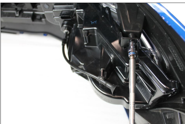
27. Carefully reinstall the accessory lamp using the OEM hardware. NOTE: Avoid contact with the Adhesive on the mounting tab.
