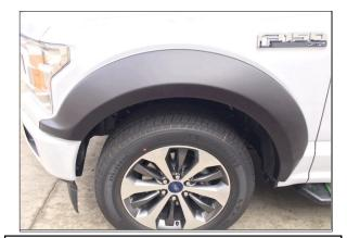
**12.** Ensure the rubber Gasket is not tucked into the Flare. If this occurs, use small plastic prying tool to fix the Gasket. Repeat Steps **1-12** on the opposite side of the vehicle.
