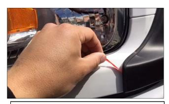
**11.** Remove the tape liner from the rubber Gasket, working from each end and meeting in the center. Firmly depress the Gasket onto the vehicle. Tighten all of the screws, final tight. Slight adjustments of the Flare position can be made while tightening for best fit.
