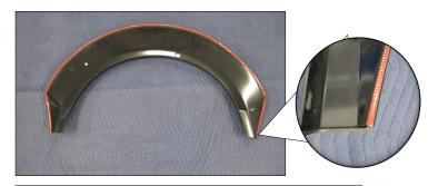
**1.** Install the Rear Gasket onto the Flare as shown, with the long sided tape edge against the inside of the Flare.
