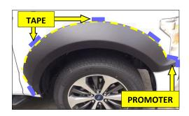
7. Dry fit the Flare onto the vehicle to familiarize yourself with the flare positioning. Note the area where the Fender Flare gasket will contact vehicle body and were the mounting blocks will contact bumper trim. Use strips of painters tape to make reference marks on fender and bumper where the Flare will be installed. Apply the Adhesion Promotor to vehicle surface at the Mounting Block location and peel the tape backer off of the Mounting Block.
