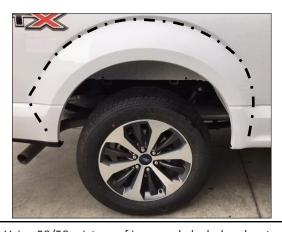
**3.** Using 50/50 mixture of isopropyl alcohol and water, clean vehicle body where Fender Flare will make contact.
