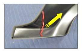
**5.** Using an O Ring pick or equivalent, pull the tape backer out of the Gasket and apply pressure to bond the gasket to the flare.
