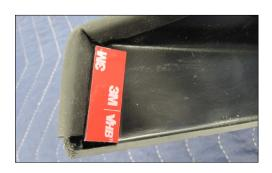
**6.** Apply Adhesion Promoter to the tip of the Flare and peel the tape backer off of one side of the Mounting block. Install the block onto the Flare as shown.
