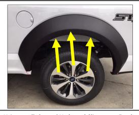
**5.** Using small channel U-shaped Clip secure Fender Flare at remaining 3 slots. Clips will snap into place when properly installed.
