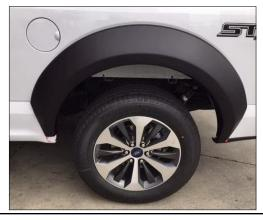
**6.** Starting at the front of the flare, remove tape liner from rubber gasket. Ensure that the Gasket is not tucking into flare. If this occurs, use small plastic prying tool to fix the Gasket. Repeat steps **1 - 4** on the opposite side of the vehicle.
