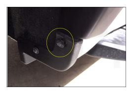
**8.** Slide the rear Fender Flare tab behind the factory mud flap. Loosely re-attach the 5.5 mm head screw to secure Flare.
