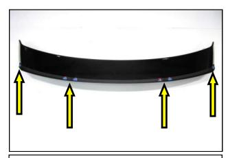
**11.** With the RTR Spoiler Lip in place, begin removing the tape backer from underneath the Lip.
