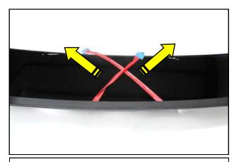
**12.** Pull the backer from each end of the strip until it is completely out from underneath the RTR Spoiler Lip then press firmly to bond the entire section of tape.
