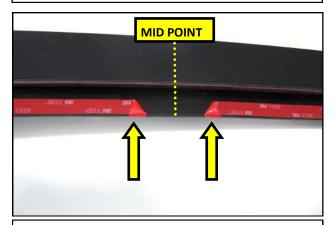
**7.** Peel approximately one inch of the backer away on each side of the cut as shown.
