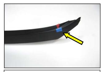
**5.** Peel and tape the backer on the outer edges of the RTR Spoiler Lip as shown.
