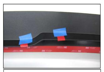
**4.** Wrap the peeled edges around the RTR Spoiler Lip and tape the edges down on the opposite side.
