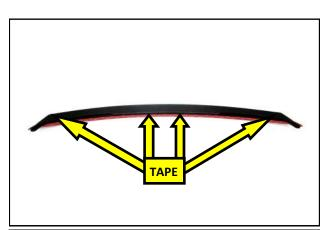
1. The RTR Spoiler Lip is intended to be installed on the trailing edge of the Performance Pack trunk spoiler. The RTR Spoiler Lip mounts to the OEM spoiler using high bond double sided tape. Proper surface preparation is very important.
