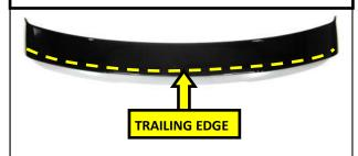
**9.** Using a mild soap and water solution, clean the OEM spoiler of any and all dirt and dust. When completely dry, wipe the top and bottom of the trailing edge using the supplied Adhesion Promoter.
