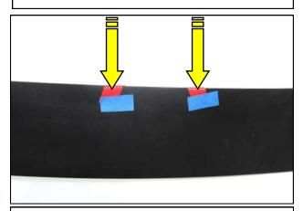
**8.** Wrap the peeled edges around the RTR Spoiler Lip and tape the edges down on the opposite side.
