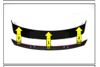
**10.** With the help of an assistant, slide the RTR Spoiler Lip onto the OEM spoiler. Firmly seat the center section first, then bring the edges in and onto the sides of the OEM spoiler. NOTE: Precise alignment is critical for a successful install.
