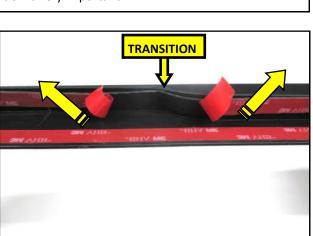
**3.** Peel approximately one inch of the backer away on each side of the cut as shown.
