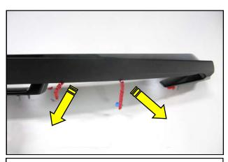
**13.** Pull the backer out from underneath the lower portion of the RTR Spoiler Lip and press firmly to bond the tape to the OEM spoiler.
