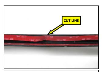
**2.** Along the upper edge, place a cut in the Tape Backer on each side approximately 1/3 of the way in, at the transition.
