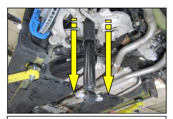
**28.** Lower the shock down into the control arm as shown, and let it hang. The shock is not to be removed.
