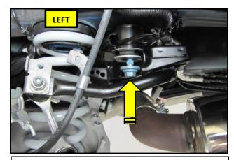
**38.** Install the side specific RTR spring into the vehicle. Start the sub frame bolts and the subframe bracket bolts. Repeat steps **50**, **51** and **52** on the opposite site of the vehicle.
