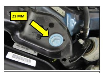
**34.** Remove the front subframe bolts on both sides of the vehicle.
