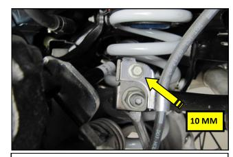
**40.** Secure the brake hose to the sway bar link using the OEM bolt.
