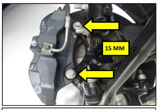
**7.** Remove the caliper anchor bolts and slide the caliper off of the brake rotor.
