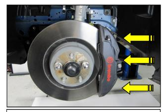
**23.** Slide the brake caliper back onto the rotor.
