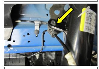
**4.** Pry the wheel speed sensor anchor out of the strut tab.
