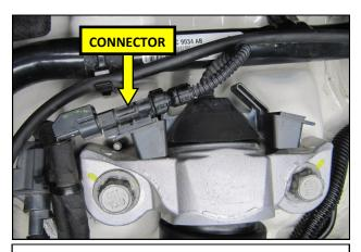
**25. REAR SPRINGS** Disconnect the MagneRide connector at the top of the shock.
