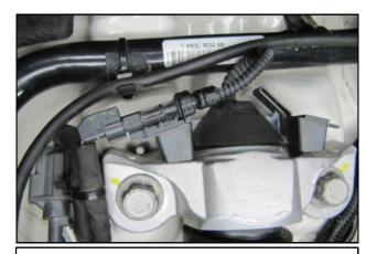
**46.** Reconnect the MagneRide harness at the top of the shock. Repeat steps **40-46** on the opposite side of the vehicle.
