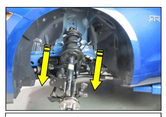
**13.** Pull the spindle away from the vehicle and remove the strut assembly.
