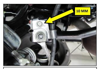
**30.** Remove the bolt securing the brake hose bracket to the sway bar. Repeat this step on the opposite side of the vehicle.
