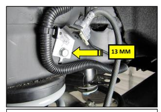
**41.** Secure the hard line bracket to the vehicle using the OEM bolt.
