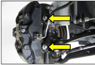
**24.**Reinstall the anchor bolts and torque them to 85 lb.ft. Repeat steps **2-24** on the opposite side of the vehicle.
