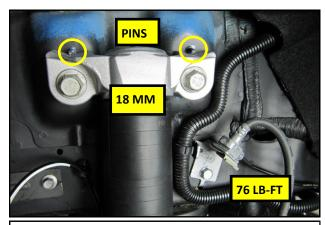
**45.** Compress the rear Shock and align the upper mount under the body alignment pins.
