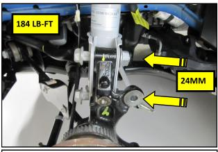
**18.** Slide the spindle into the strut and re install the strut-to-spindle bolts and nuts. Torque the fasteners to 184 lb.ft.
