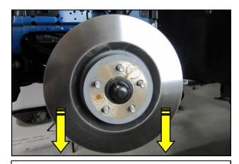
**9.** Slide the brake rotor off of the hub and set it aside.
