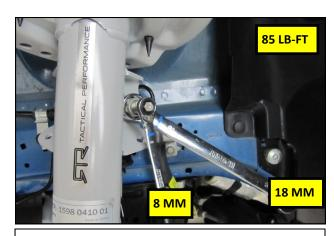
**20.** Insert the front sway bar link into the RTR Strut tab and re use the OEM nut to secure it. Torque the link nut to 85 lb.ft.
