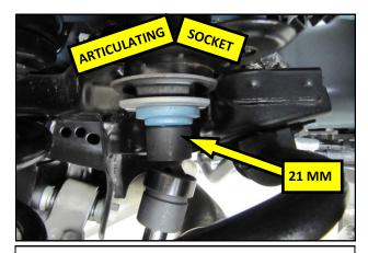
**35.** Using a 21 mm Articulating socket, remove the rear subframe bolts on both sides of the vehicle and lower the differential and subframe until the springs can be removed.
