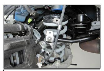
**37.** Transfer the OEM isolator onto the RTR Spring. Rotate the isolator in the spring until the coil end bottoms against the isolator
