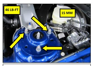
19. Torque the upper strut nuts to 46 lb.ft.
