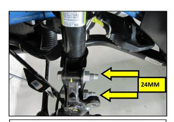
10. Remove the strut to spindle nuts.
