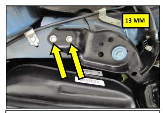
**33.** Remove the subframe bracket bolts on both sides of the vehicle and set them aside.
