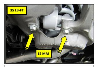
**44.** Install the lower Shock bolts. Torque the bolts to 35 lb.ft.
