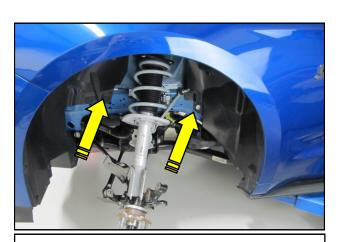
**16.** Lift the Strut assembly into the vehicle and align the studs with the holes in the strut tower.
