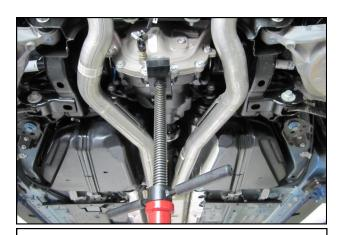
**32.** Support the differential using a jack as shown.
