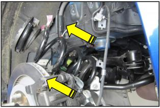
**36.** Remove the OEM spring and upper isolator from the vehicle.
