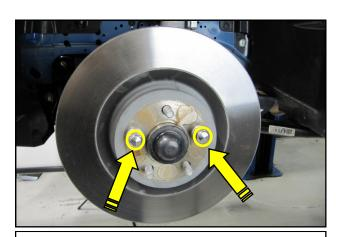
**22.** Slide the brake rotor back onto the hub and secure it using two lug nuts.
