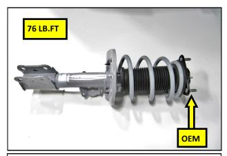
**15.** Compress the RTR Spring and reuse the OEM strut mount and nut from step **14** to build the assembly. Torque the strut nut to 76 lb.ft.
