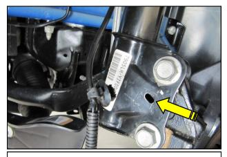
**5.** Pry the second wheel speed sensor anchor out of the strut mount.
