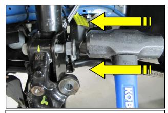
**11.** Reinstall the nuts, flange side out until flush with the bolt. Using a 5 Lb. sledge hammer, carefully drive the bolts out of the spindle. Remove the bolts and nuts and set them aside.
