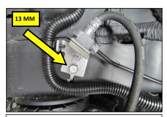
**29.** Remove the bolt in the hard line bracket and set it aside. Repeat this step on the opposite side of the vehicle
