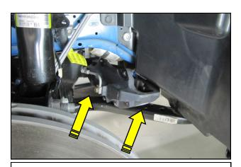
**8.** Slide the caliper up onto the K member or support it using a suitable strap.
