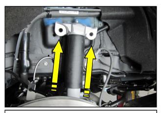
**43.** Raise the shock out of the lower control arm.
