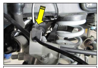
**42.** Insert the wheel speed sensor wire into the parking brake cable bracket.
