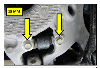
**27.** Remove the lower shock bolts in the control arm and set them aside.
