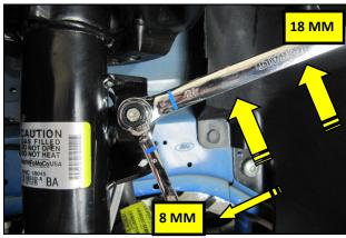
**6.** Disconnect the sway bar link from the strut as shown.
