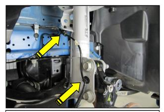
**21.** Insert the wheel speed sensor wire anchors into the Strut a shown. Reconnect the MagneRide harness, ride height sensor, and the brake hose.
