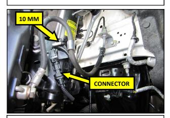
**3.** Using a 10 mm socket, Unbolt the brake hose bracket from the strut body. Disconnect the MagneRide harness at the bottom of the strut.
