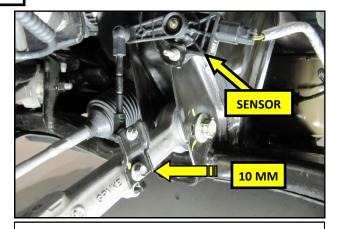
**2. FRONT SPRINGS** Using a 10 mm socket, disconnect the ride height sensor from the control arm.
