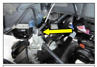
**31.** Slide the wheel speed sensor wire out of the parking brake cable bracket. Repeat this step on the opposite side of the vehicle.
