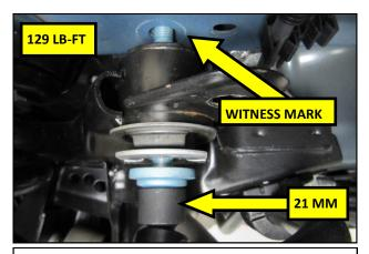
**39.** Use a pry bar to guide sub frame while tightening the subframe bolts. Align the subframe mounts with the witness mark in the vehicle. Torque the bracket bolts to 41 lb.ft. Torque the subframe bolts to 129 lb.ft.
