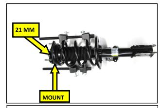
**14.** Compress the OEM spring in the strut assembly until the tension is fully relieved. Remove the nut and upper strut mount and set them aside.
