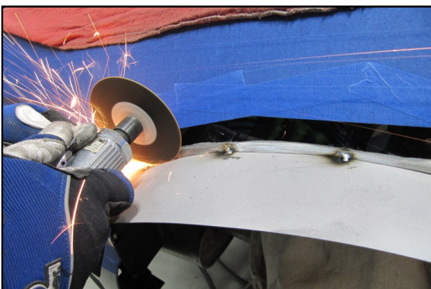
23. Using a cut of wheel, trim the excess Fender Extension off of the vehicle. NOTE: Depending on your inner fender cut, you may have excess material to remove at one or both ends of the extension.
