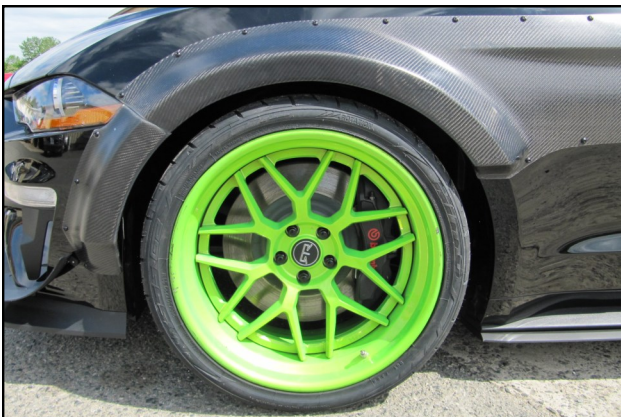
53. Reconnect the battery. Mount the wheels and tires and check clearance at full lock, left and right and test drive to check clearance under compression.
