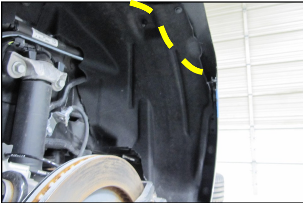
35. Trim the rear of the fender liner to gain sufficient wheel and tire clearance.
