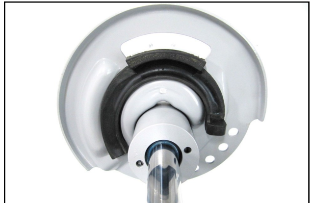
14. Transfer the Coil isolator from the OEM into the RTR Strut as shown.
