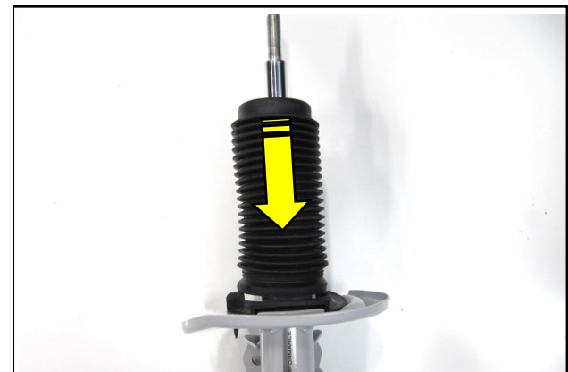
16. Install the boot onto the Strut.
