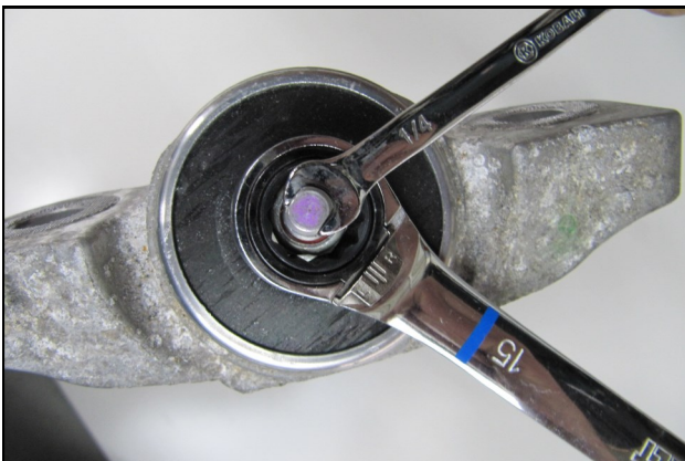
31. Remove the upper shock lock nut and mount.
