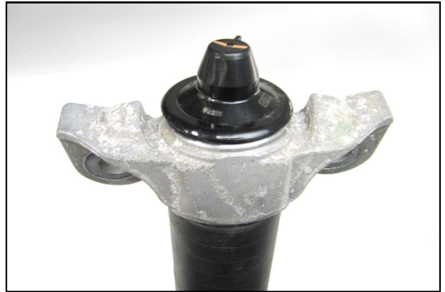
30. Remove the debris cap from the upper shock mount.
