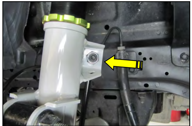
20. Insert the Sway Bar Link into the RTR Strut tab and use the supplied Nut to secure it. Torque the Link Nut to 85 lb.ft.
