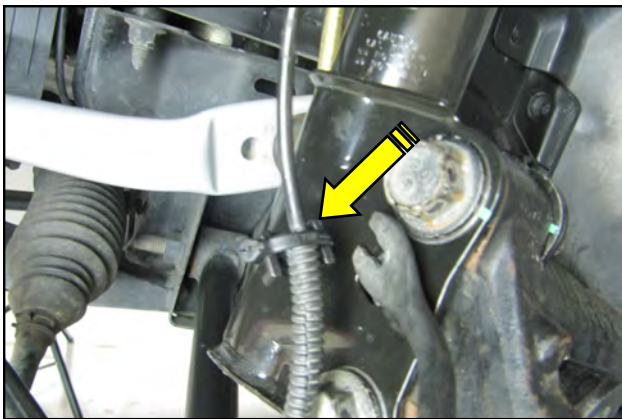
3. Pry the second wheel speed sensor anchor out of the strut mount.
