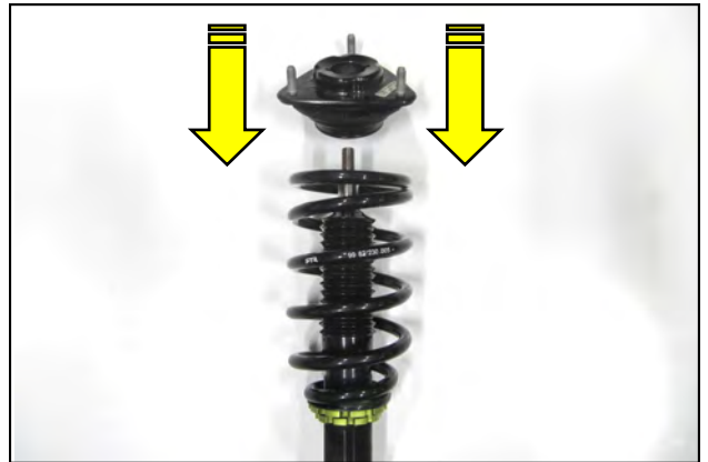
14. Transfer the OEM upper strut mount and bearing onto the RTR Coilover assembly.
