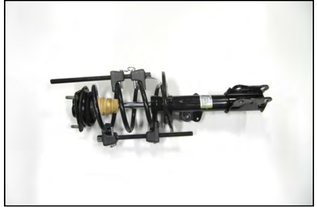
12. Compress the OEM spring in the strut assembly until the tension is fully relieved.
