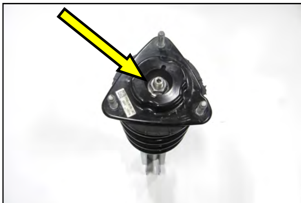
15. Use the supplied Nut to secure the mount and bearing onto the piston rod and torque to 26 lb.- ft.
