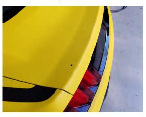
**Step 5:** Wipe the tape surfaces on the deck lid panel with the provided alcohol wipes. Then test fit the spoiler to confirm fitment.
