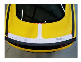
**Step 3:**Using the aligned template, mark and drill 1/8" pilot holes. Finish with a 3/8".
