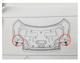
**Step 2:** Close the trunk and align the supplied template with the front and sides of the deck lid.
