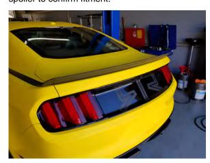
**Step 6:**Remove the tape backing and apply the supplied adhesion promoter. Allow time for the adhesion promoter to flash dry.
