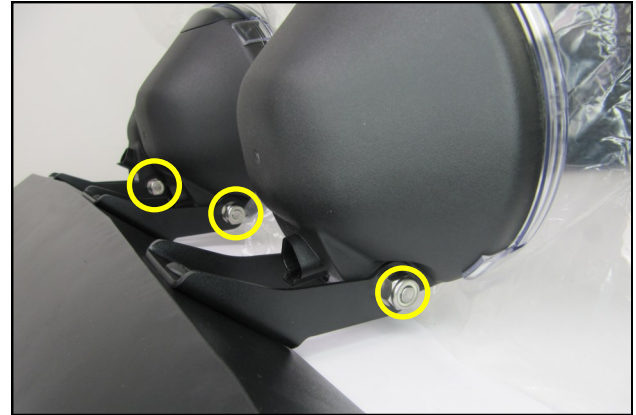
35. Slide the lights into the RTR Light Brackets as shown and secure them using the hardware removed in step 33. Leave the mounting hardware snug at this time.
