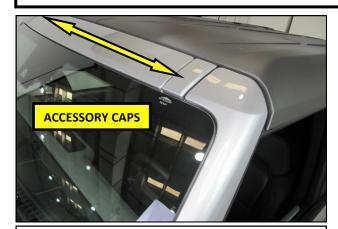
**1. Disconnect the Negative battery terminal.** Using a plastic trim removal tool, pry off both of the accessory caps and set them aside.
