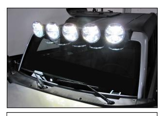
**40.** Reconnect the Negative battery terminal and perform a function check based on the option chosen. Standard Broncos will use Aux. switch number One and Bronco Raptors will use switch number Three for light actuation.
