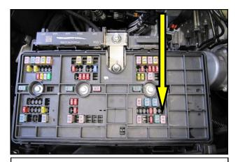
**49. NOTE:** The number **60**, 30 amp fuse in the under hood fuse box protects the light Bar circuit.
