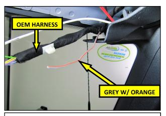
**22.** INSTALL OPTION ONE: The Locate the Grey wire with the Orange tracer looped into the OEM harness
