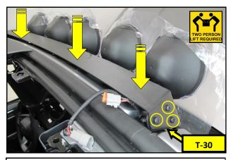
**38.** With the help of an assistant, lower the Light Bar assembly onto the Light Bar Brackets. Check the Wire Harness to roof clearance and reroute if necessary. Secure the Bar on each side using the 6mm Button Head Bolts. Leave the bolts snug for now.
