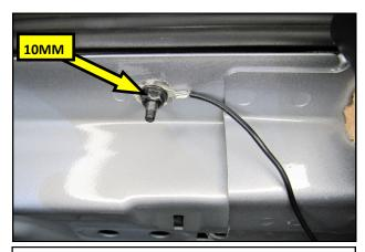
**19.** Reinstall the bolt from step **17**. and slide the Ring Terminal on the black wire onto it. Secure the Ring Terminal using the OEM nut. Do not over tighten.
