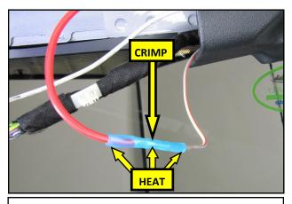
**23A.** INSTALL OPTION ONE: Strip approximately 3/16" of insulation from the Red wire in the RTR Pig Tail and from the Grey/Orange accessory wire and use the supplied Butt Connector to crimp the two together. Using a heat gun on low, shrink the insulation down onto the wires.
