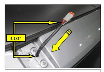
**14.** Insert the taped end of the Pig Tail into the hole drilled in step **11.** Leave approximately 3 1/2" of the Pig Tail outside of the vehicle. **Use the supplied silicone adhesive/ sealant to seal the hole drilled in step 12.**
