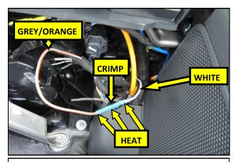
**24.** In the passenger side footwell, locate the other end of the Grey accessory wire with the Orange tracer looped into the OEM harness and pull the free end out. Locate the White accessory wire taped to the harness. Using the supplied Butt Connector- Strip, crimp and heat shrink the two wires together.
