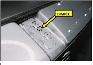
10. On the passenger side of the roof, locate the dimple between the accessory cap studs and drill a 1/8 " pilot hole.
