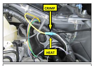
**27.** Using the supplied Butt Connector- Strip, crimp and heat shrink the two wires together. Secure the wires using the last Cable Tie. Use electrical tape to wrap the wires if needed.
