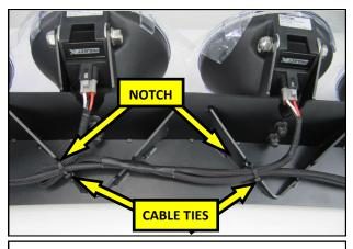
**37.** Secure the Harness to the Light Bar using the Edge Clip Cable Ties. Slide the clip into the notch in the Bar support and cinch the Tie down onto the Harness'. Trim the excess length.
