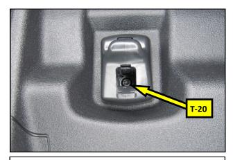
**7.** Using a T-20 TORX® driver remove the screw inside of the visor clip and remove the clip. Repeat steps **3-7** on the opposite side of the vehicle.
