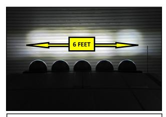
**48.** With the vehicle parked on level ground, 10 feet from a vertical wall, adjust the lights to the desired beam pattern and tighten the bolts final tight. RTR recommends starting by adjusting the center of the beams to a height of 6 feet. **NOTE:** Tire size and suspension options will have an effect on this measurement.
