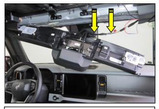
**42.** Reconnect the wiring harness to the windshield trim panel.
