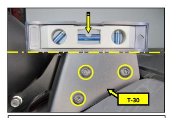
**47.** With the vehicle parked on level ground, place a level on the top of the Light Bar as shown. Adjust the angle of the Light Bar as needed to get it parallel to the ground. Tighten all six light Bar screws, final tight.
