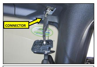
**5.** Release the sun visor from the roof and disconnect the wiring harness. Set the visor aside for now.
