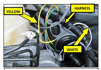
**26**. Under the hood, at the driver side firewall, locate the Yellow and white accessory wires taped to the OEM harness and unwrap them.
