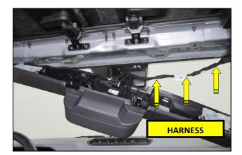
**9.** Having all 4 panel clips released, unclip the wiring harness from the panel.
