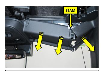
**8.** Starting at the panel seam, pull down and release the clips securing the windshield trim panels a shown.
