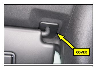
**3.** Starting at the passenger side of the vehicle, Use a plastic trim removal tool to pry off the sun visor screw cover.
