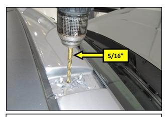
**11.** Using a 5/16" drill bit, enlarge the pilot hole in the roof.
