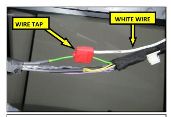
**21.** <u>INSTALL OPTION ONE:</u> Using the supplied Wire Tap, connect the White RTR Pig Tail wire to the Green wire
