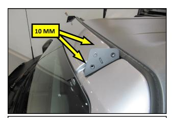
**30.** Install the Driver side Light Bar Bracket onto the vehicle a shown, using the OEM nuts removed in step **2.** Leave the nuts sung at this time.
