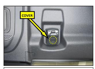
**6.** Using a pocket screwdriver, or equivalent, pry open the screw cover in the sun visor clip.
