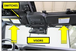
**45.** Reinstall the visors removed in step **5. NOTE:** The Driver side visor has the 3 button switch panel.
