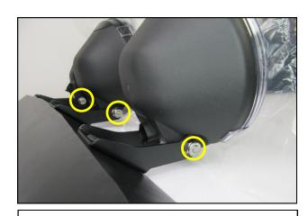
**35.** Slide the lights into the RTR Light Brackets as shown and secure them using the hardware removed in step **33**. Leave the mounting hardware snug at this time.
