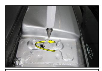
**12.** Using a deburring tool, remove all of the sharp edges in the sheet metal. Clear the hole of any remaining debris.
