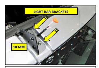
**29.** Install the Passenger side Light Bar Bracket onto the vehicle a shown, with the Connector half of the Pig Tail pointed towards the Drivers side of the vehicle. Secure the Bracket using the OEM nuts removed in step **2**. Leave the nuts sung at this time.
