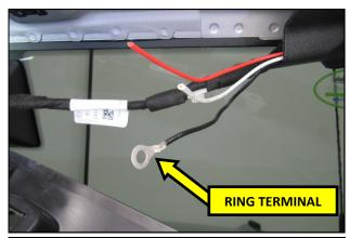
**16.** Strip approximately 3/16" of insulation from the Black wire and crimp the supplied Ring Terminal onto it.
