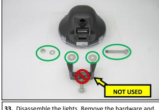
**33.** Disassemble the lights. Remove the hardware and mounting bracket. Set the bracket and short bolt aside. They will not be used with the RTR Light Bar.
