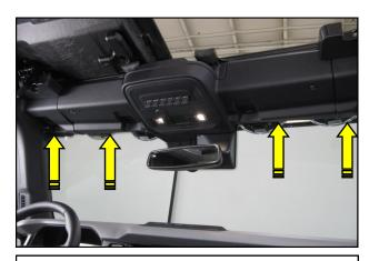
**43.** Reinstall the trim panels and check for any untucked wiring.
