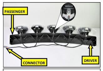
**36.** Turn the Light Bar assembly upside down on a protective work surface and connect the Harness to the Lights. When properly installed, the Connector will be on the Left with the Lights facing away.
