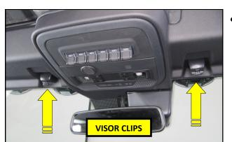
**44.** Reinstall the visor clips removed in step **7**. Do not over tighten.
