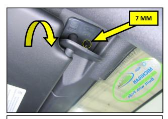
**4.** Rotate the screw cover to gain access to the visor screw. Using a 7 mm socket, remove the screw.
