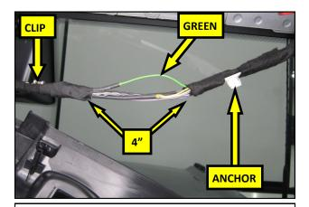
**20. INSTALL OPTION ONE:** Unwrap approximately 4" of the OEM wire harness between the metal trim clip and the plastic anchor to expose the wires. Locate the Green wire and separate it from the other wires.
