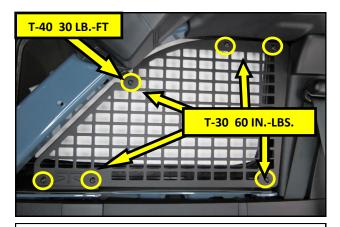
**9.** Using a T-30 TORX<sup>®</sup> driver and the supplied M6 Bolts, secure the RTR MOLLE Plate to the Brackets. Torque the fasteners to 60 in.-Lbs. Adjust the Mid Bracket if needed, and Torque the Bracket Bolt to 30 Lb.-Ft. Reinstall the remaining OEM hard top hardware.
