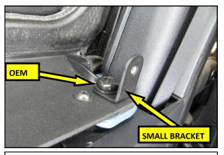
**5.** Install the Small Bottom Bracket a shown, using the OEM hardware . Torque the bolts to 106 in.- lbs.
