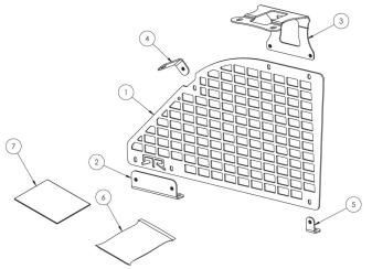
**Components Included MOLLE** Plate 1. 1 2. Large Bottom Bracket 1 3. Top Bracket 1 4. Mid Bracket 1 5. Small Bottom Bracket 1 Hardware Pack 6. 1 7. Instructions 1
