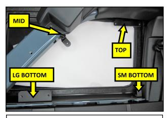
**8.** Locations of all 4 brackets when properly installed in the vehicle.
