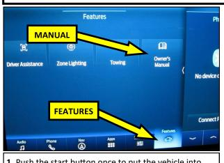
1. Push the start button once to put the vehicle into Accessory mode and select Features, then Owner's Manual in the center display.
