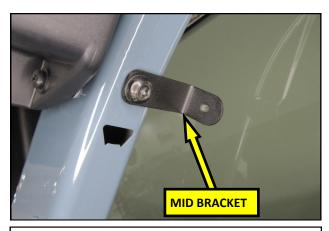
**7.** Using the third supplied M8 Bolt, mount the Mid Bracket to the vehicle as shown. Leave the Bolt loose to allow for final adjustment.
