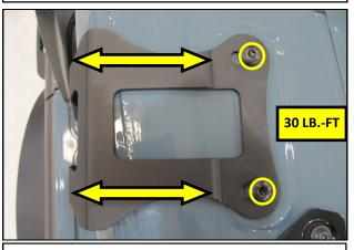
**4.** Using two of the supplied M8 Bolts, mount the Top Bracket to the roof as shown, with sufficient clearance between the bracket and vehicle. Using a T– 40 TORX<sup>®</sup> driver, torque the Bolts to 30 Lb.-Ft. Return the top onto the vehicle but do not secure it with the hardware.
