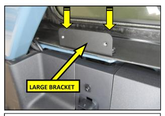
**6.** With the top on the vehicle, install the Large Bottom Bracket a shown using the OEM hardware. Torque the bolts to 106 in.- lbs.
