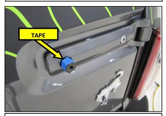
**4.** Wrap the Adapter Nut with a protective layer of painters tape or equivalent.
