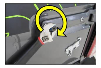
**5.** Using an adjustable wrench, snugged down onto the wrapped Nut, tighten the Adapter Nut to approximately 30 Lb. Ft. If need be, the tape can be removed and torque wrench with a 20 MM socket can be used.
