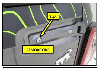
**2.** With the tailgate closed, use a T-45 TORX<sup>®</sup> driver to remove one hinge bolt from the tailgate.
