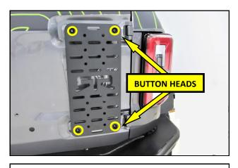
**8.** Completed install showing the RTR MOLLE Accessory Plate on the OEM tailgate hinges using the Adapter Kit.
