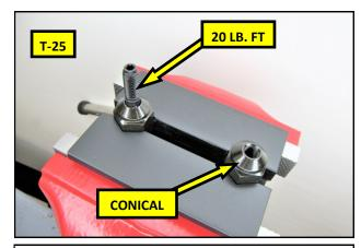
1. Place the Adapter Nuts into a soft jawed vice, conical side up, and thread the M8 Studs into them. Using a T-25 TORX<sup>®</sup> driver, torque the Studs to 20 Lb. Ft. Install the Studs into al four of the Adapter nuts.
