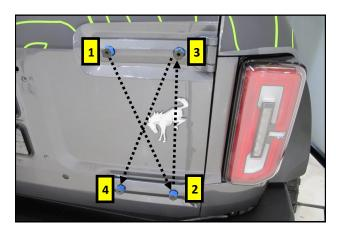
**6.** Repeat steps **2-5**, one at a time for the three remaining hinge bolts in an alternating pattern. Remove the tape when complete.
