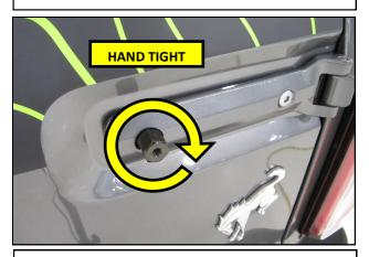
**3.** Thread the Adapter Nut with stud into the bolt hole from step **2** hand tight.
